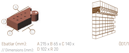
Silme Pres Tuğla // Special Radial Lintel Facing Brick
